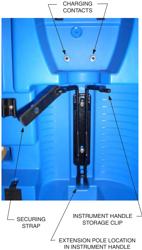
Fig 12.21 Charging Station - Instrument Location
