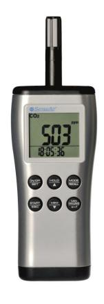
**psense** II ™ is a hand-held and portable data logger, with rechargeable batteries and power adaptor. The instrument displays and records temperature, relative humidity, CO<sub>2</sub>, and calculates parameters such as dew point and wet-bulb temperature. **psense** II ™ can be run in different modes such
